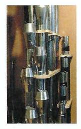
Our pipes are the best made in the world. We use thick high tin-content pipe metal rather than zinc in our flues and reeds (as well as wood and copper), and support them in felt-lined traces which prevent the pipes from collapsing.
